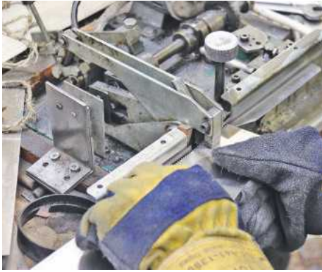
▲ Here the standard handsaws are hand fed through the setting machine
